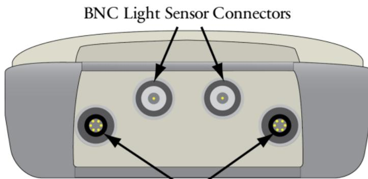
LAI-2250 Optical Sensor (wand) connectors X and Y
