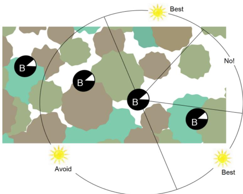
*Figure 5-3. Measurement direction with direct sun. In gapped or isolated canopies, if you are measuring with the sun out and doing scattering correction, try to keep the sun to the side or a bit in front. Avoid having the sun behind you, especially if it is lower in the sky.*
