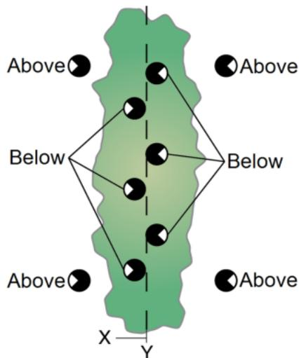
Next, characterize the canopy shape by measuring a number of X, Z coordinates. The number of coordinates required will vary, depending on the complexity of the canopy shape. If the canopy is asymmetrical, characterize each side with X, Z coordinates. Measure or estimate the row ratio for the hedge (the length Y over width X). These values are used by FV2200 software to compute the foliage density or dripline LAI.
