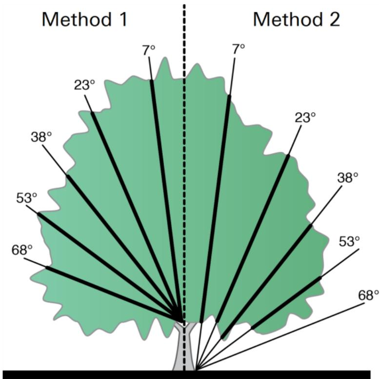
The thick segments of the diagonal lines in this figure indicate the distances each ring sees through the canopy. Note that sometimes a ring will see no foliage, as with the 68° ring in Method 2 above. A ring that sees no foliage should be masked. A 90° or 45° view cap can be used to further reduce the size of the canopy that is sampled. The view cap and view directions should be chosen to avoid including neighboring trees in the measurement.
