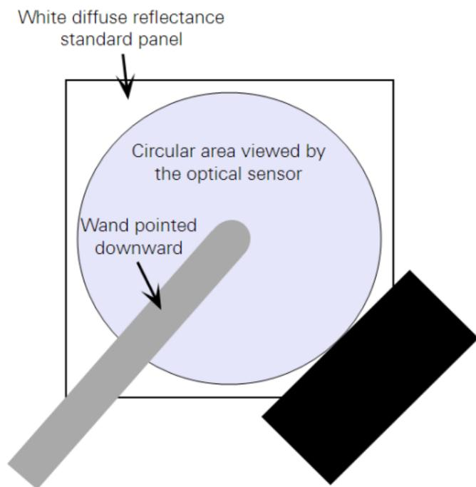
*Figure 8-1. Determining wand height for measuring leaf optical properties. Viewed from above. Shade three corners of the reflectance panel to determine the area viewed by the optical sensor. Shading of the viewed area causes the reading to change. Adjust wand height until the viewed area fills as much of the reflectance panel as possible without getting very close to the edge.*
