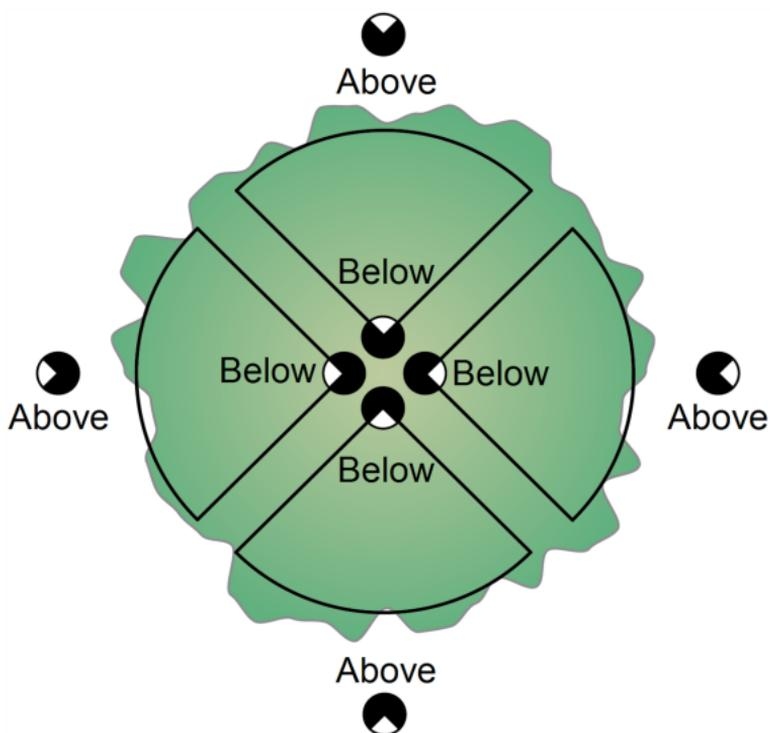
If a tree is asymmetric, then the path lengths through the tree (and thus the distance vector) will depend on azimuthal direction. Since only one distance vector is associated with a file, asymmetric trees should be measured using several files. Average foliage density is then computed by averaging the foliage densities from each of the files.
