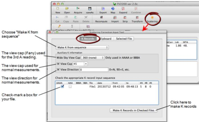
Once the K records are made, the "Records" field in the main view will show the change (Added 1 K, 'removed' 3 As).
