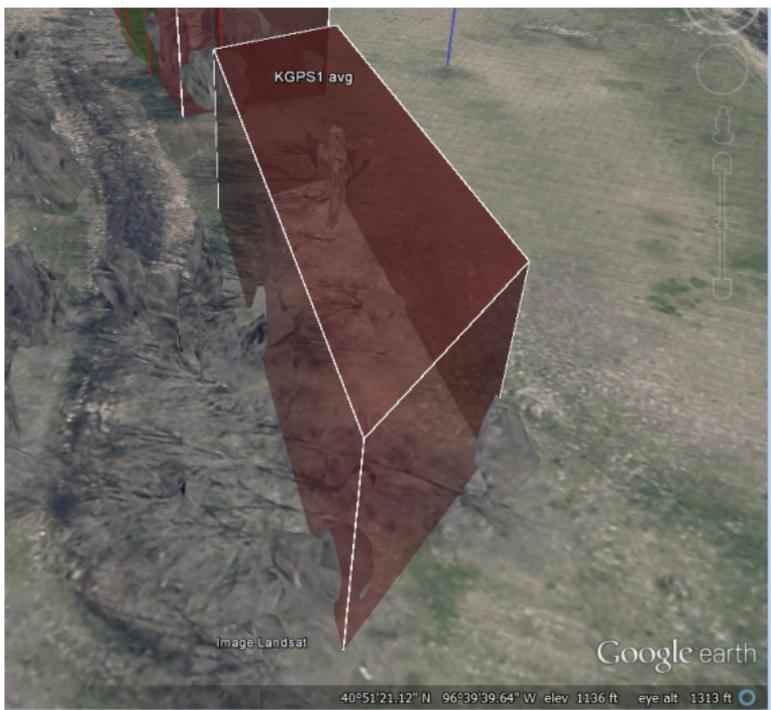
*Figure 3-2. Plot marked by GPS Tagging. At each corner of the plot, the "1" key was pressed while a file was open to log a GPS record. A different numeric key could be used to mark other plots in the same file.*
