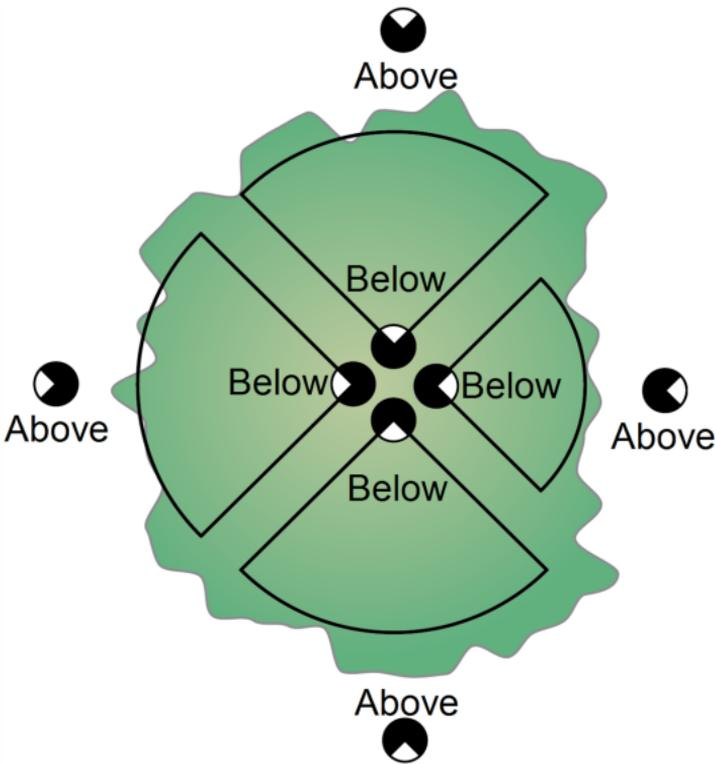
A simple method for computing path lengths and canopy volumes is provided in the FV2200 software. Use a coordinate system centered below the tree, and determine the coordinates of a sufficient number of points to describe the shape of the canopy. Alternatively, a photograph of the tree that includes a meter stick for scale can be used to obtain the tree profile.
