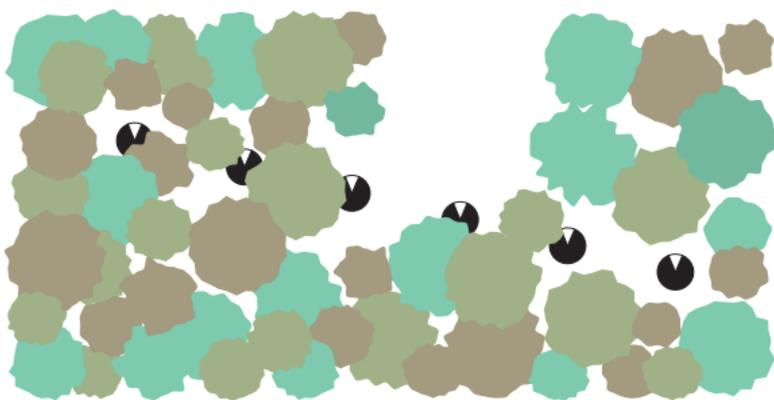
The Canopy Gap Test (see *The Gap Test* on the facing page) can be used to estimate the error of using a wide field of view in a heterogeneous canopy, when large gaps and foliage are included in the same **B** reading.
