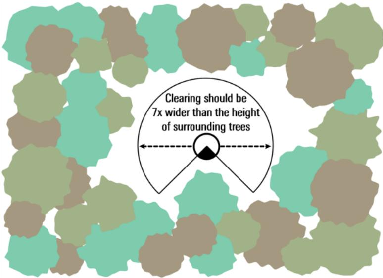
With the  $90^\circ$  or  $45^\circ$  view cap, however, a clearing half that size (diameter only 3.5 times the tree height) can be used, since the sensor can now be positioned on the edge of the clearing (looking in).
