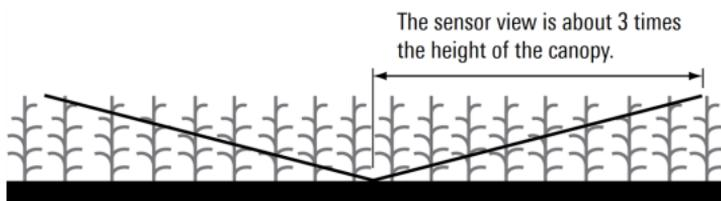
In a canopy that is 1 m high, the optical sensor should be at least 3 m from the edge in any direction that it can “see”. In a plot so small that the sensor will “see” outside the plot area if measured from the middle, one could use a 90° view cap and make readings from the corners looking into the plot. Alternatively, a 180° view cap could be used if the measurements were taken near the center of the plot.
