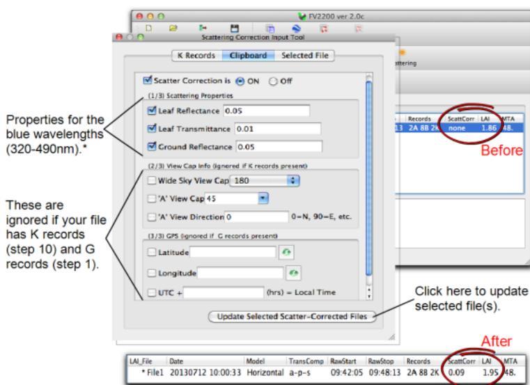
*Figure 8-3. Clipboard for scattering correction inputs. For information on obtaining scattering properties, see Required Inputs for the Scattering Model on page 10-13.*
