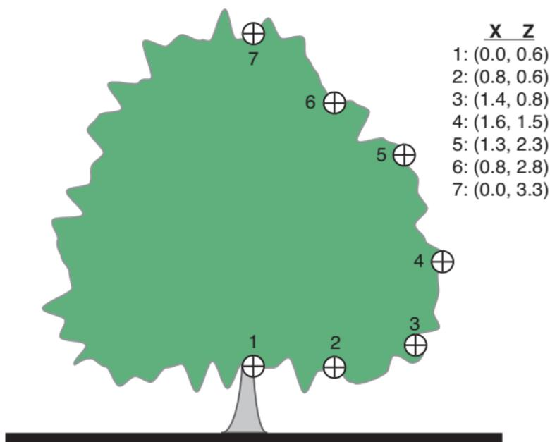
The FV2200 software can use these data to determine path lengths, neglect rings if necessary, and compute canopy volume, foliage density, or dripline LAI.
