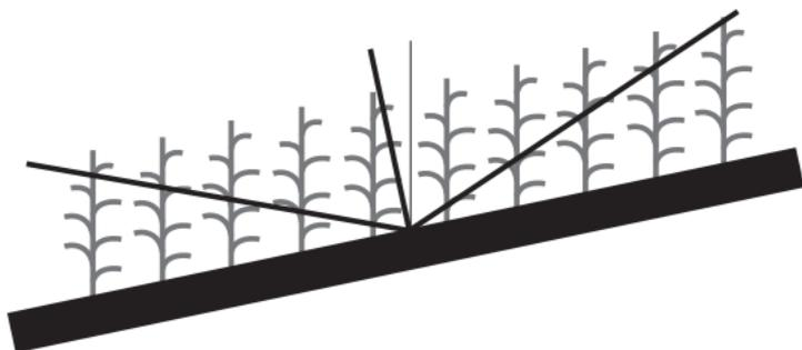
*Figure 4-1. Tilt the sensor to match the slope.*
