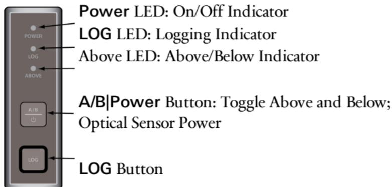
Optical sensors will turn on when the control unit is turned on (if the wand and control unit are attached), when the optical sensor cable is connected to a powered-on control unit, or when the optical sensor power button is pressed (when disconnected from the control unit). To turn the optical sensor off, press and hold the **A/B|Power** button for 2 seconds. To switch between **A** and **B** readings press and release the **A/B|Power** button.
