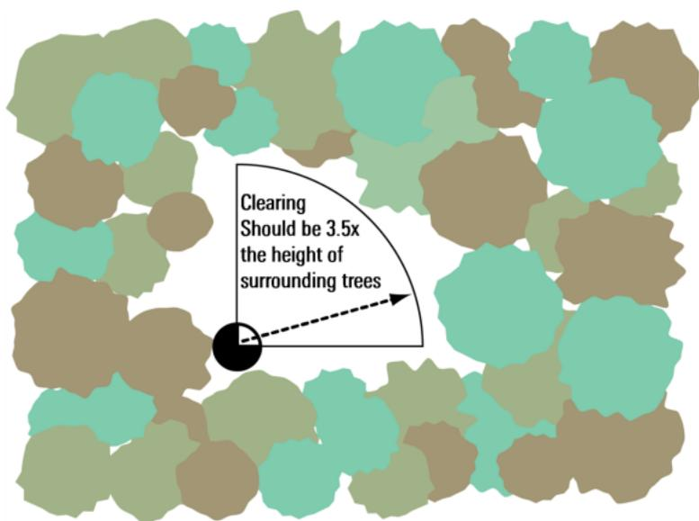
This is a common reason for using a narrow view cap in a forest. Neglecting the outer ring may be necessary if an adequately large clearing is not available. In that case, the clearing should be 1.5 times the canopy height if the 45° or 90° view cap is used. Refer to the *Small Plots* on page 6-1.
