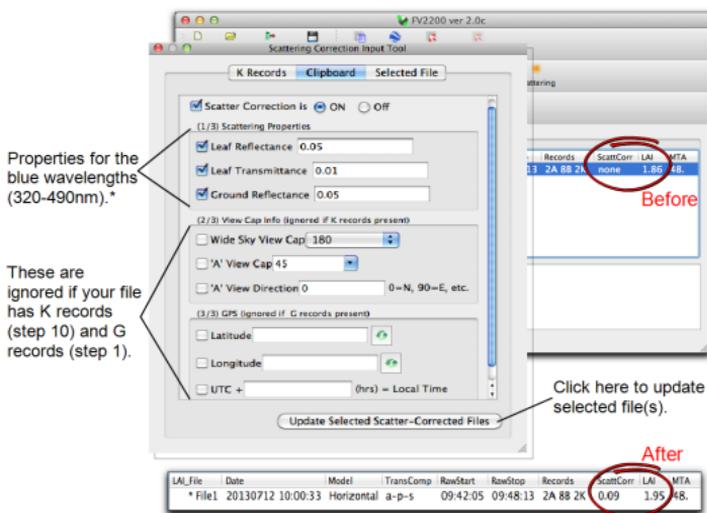
The file is now corrected for scattering, and the LAI increased from 1.86 to 1.95.
